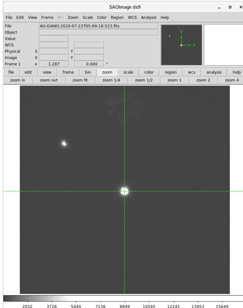
Figure 13. The Sequencer SAOImage ds9 window showing an AG acquisition image.
