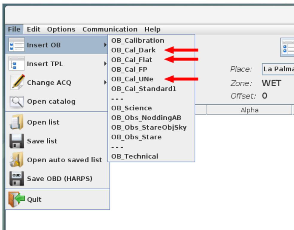
Figure 28. NSTS GUI part. The menu items with Calibration OBs are shown with the arrows.
