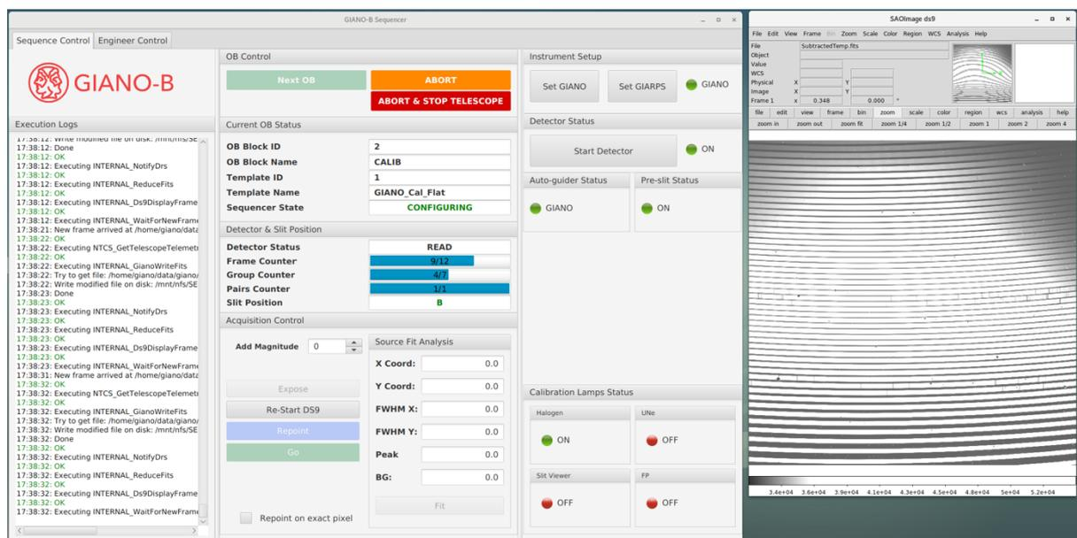
Figure 30. Sequencer GUI during Flat calibration exposures.
