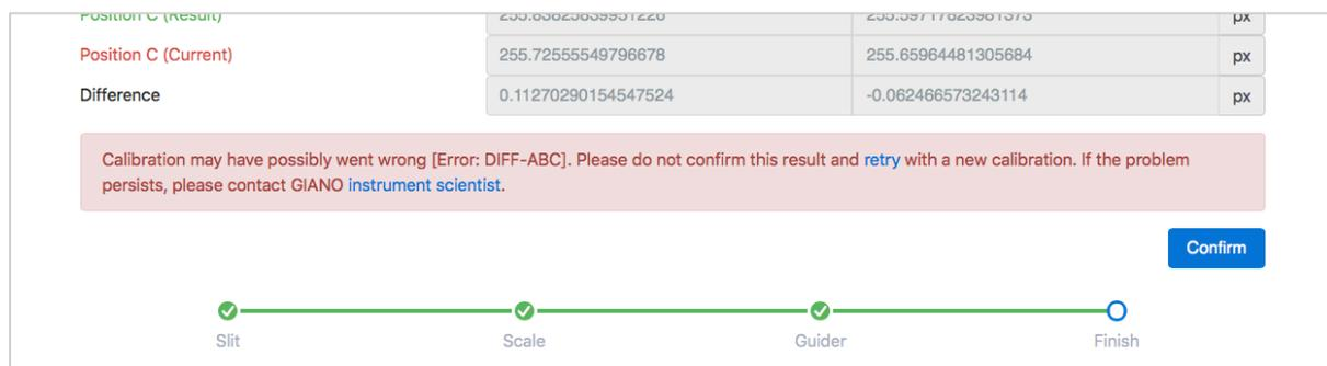
Figure 33. Slit auto-calibration results page part with a warning message.
