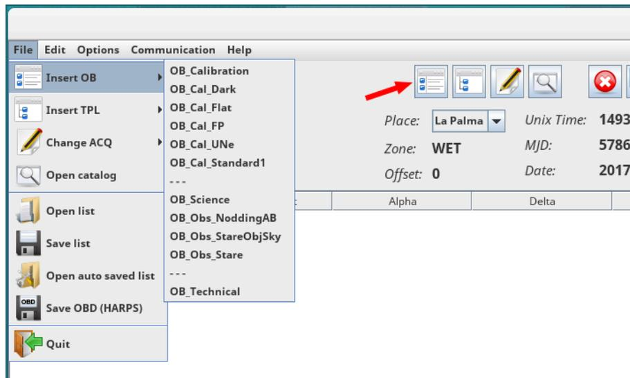
Figure 14. NSTS GUI part. Insert OB command of the menu with available OB selection, and with the red arrow indicating Insert OB shortcut.
