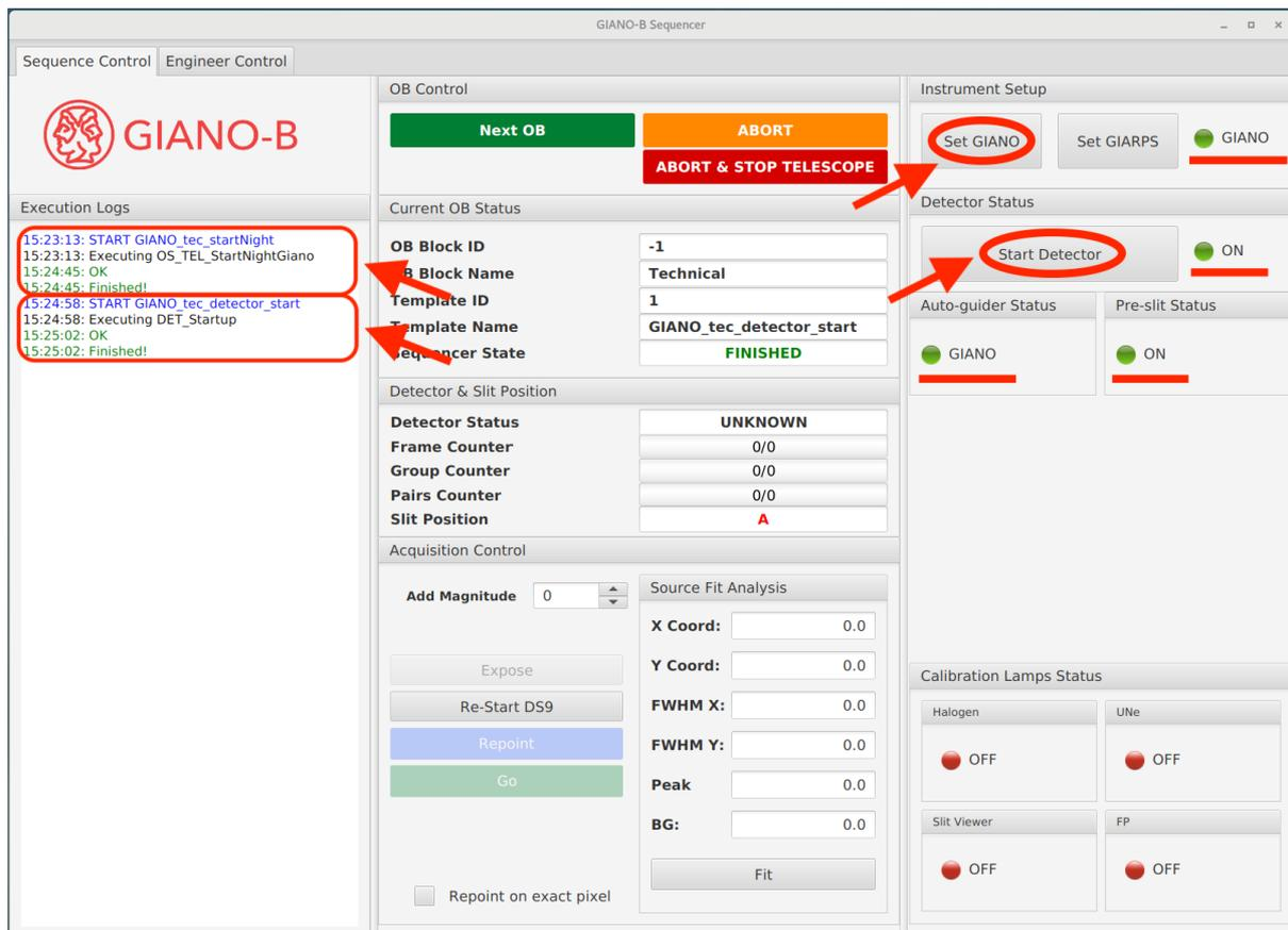
Figure 9. The Sequencer GUI with buttons used for initialization and corresponding status leds and log messages indicated in red.
