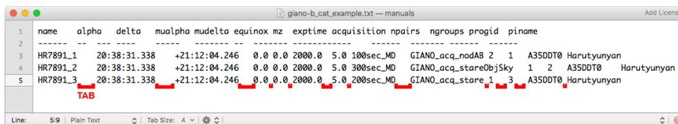
Figure 18. An example catalog in a text editor window with the tabs indicated in the last row.
