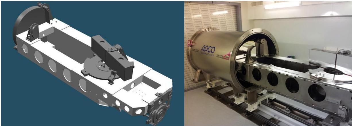
Figure 1 – HARPS-N mechanical design and vacuum vessel
