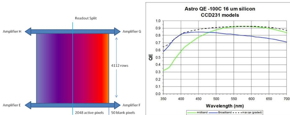
Figure 8 – The CCD coating and quantum efficiency
