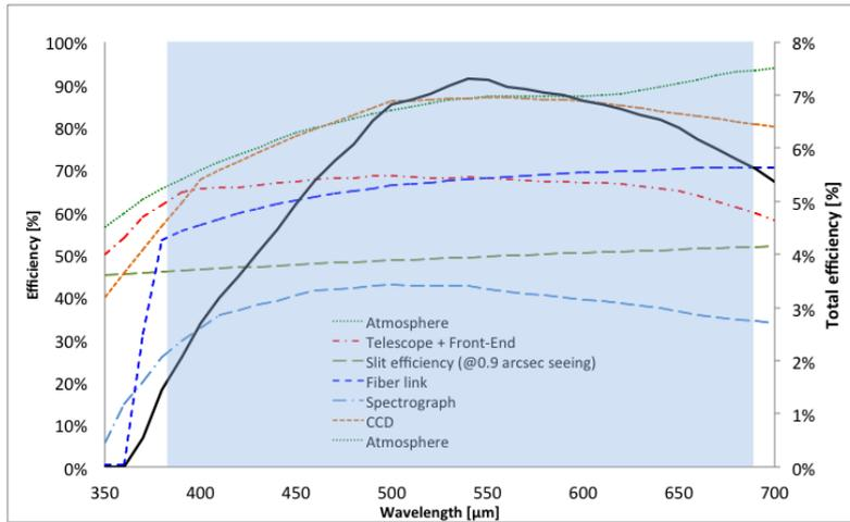
**Figure 18 - Total efficiency of HARPS-N (black plain curve, right-hand scale), and efficiency of subsystems (left-hand scale). The values have been calculated for each echelle order at its blaze wavelength. The fast drop below 380 nm is produced by a band-pass filter installed in the fiber-link to remove 2<sup>nd</sup>-order of the grism. The grey area shows HARPS-N' spectral range.**
