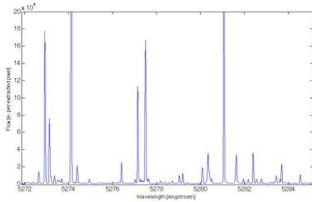
Figure 16 - Portion of the extracted ThAr spectrum order
