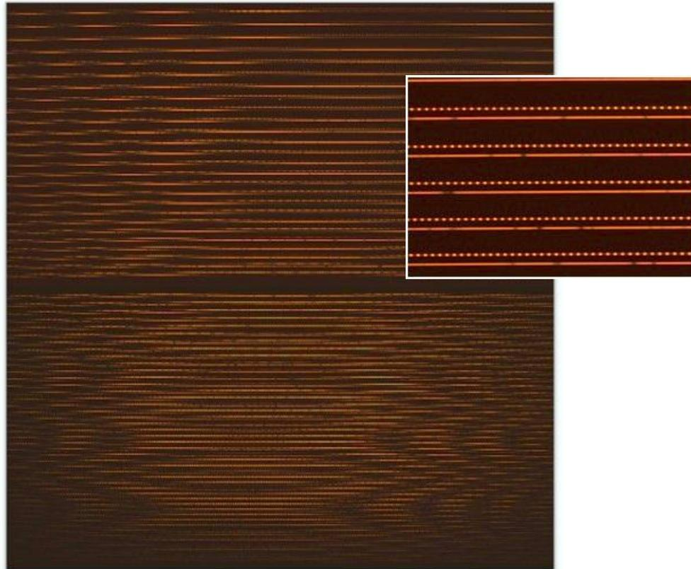
Figure 17 - Raw of a spectrum recorded by HARPS in the 'wave' mode. Two spectra can be distinguished, each one corresponding to one spectrograph fiber illuminated by A) the star (lower fiber) and B) the simultaneous FP (upper fiber).
