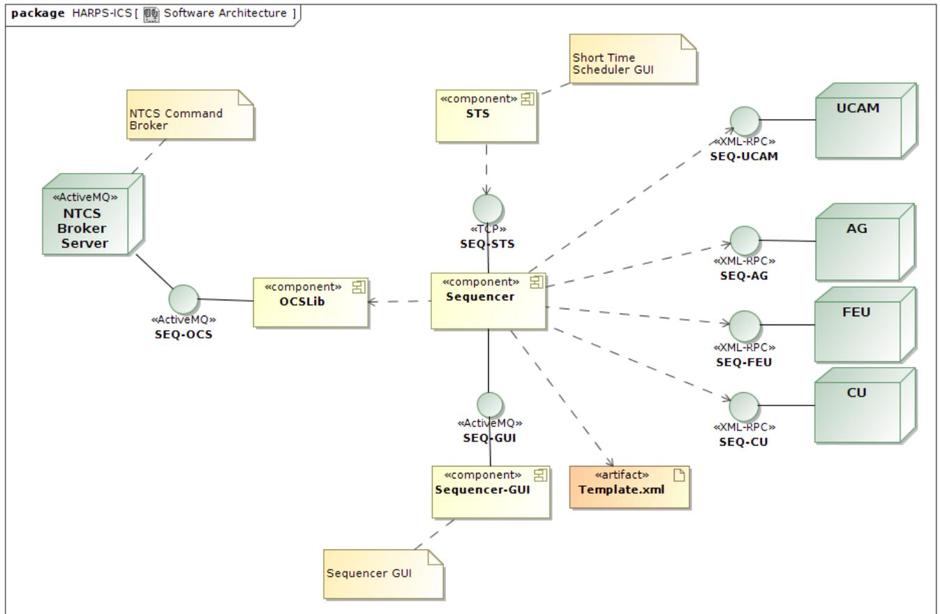
Figure 9 - The HARPS-N software architecture
