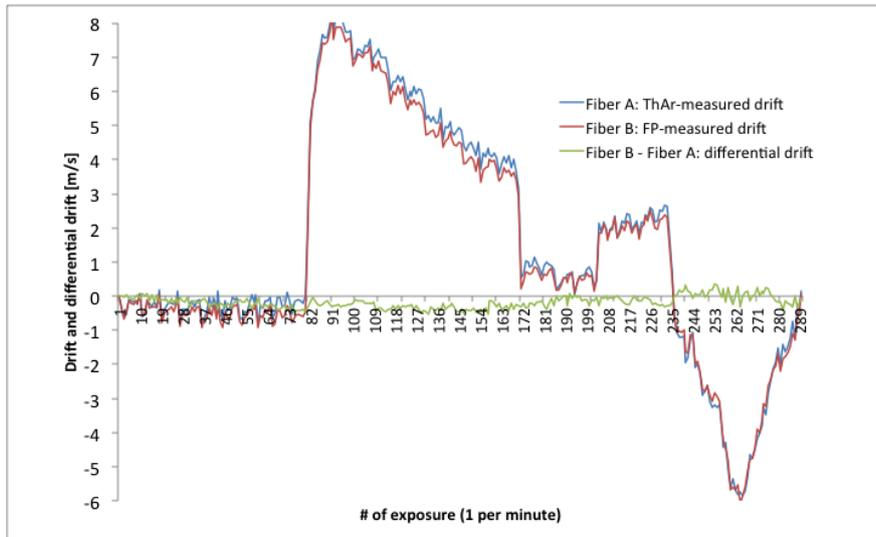
Figure 20 -Short-term stability of the spectrograph and quality of the FP and ThAr tracking technique
