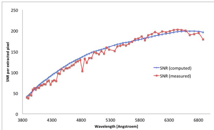
Figure 19 - Measured signal-to-noise ratio SNR of HARPS-N (red curve) compared with the values computed by the exposure-time calculator of the STS (blue curve). The efficiency tests have been carried out on HD 127334, a  $m_v = 6.36$  G5 star. The exposure time was of 120 seconds.
