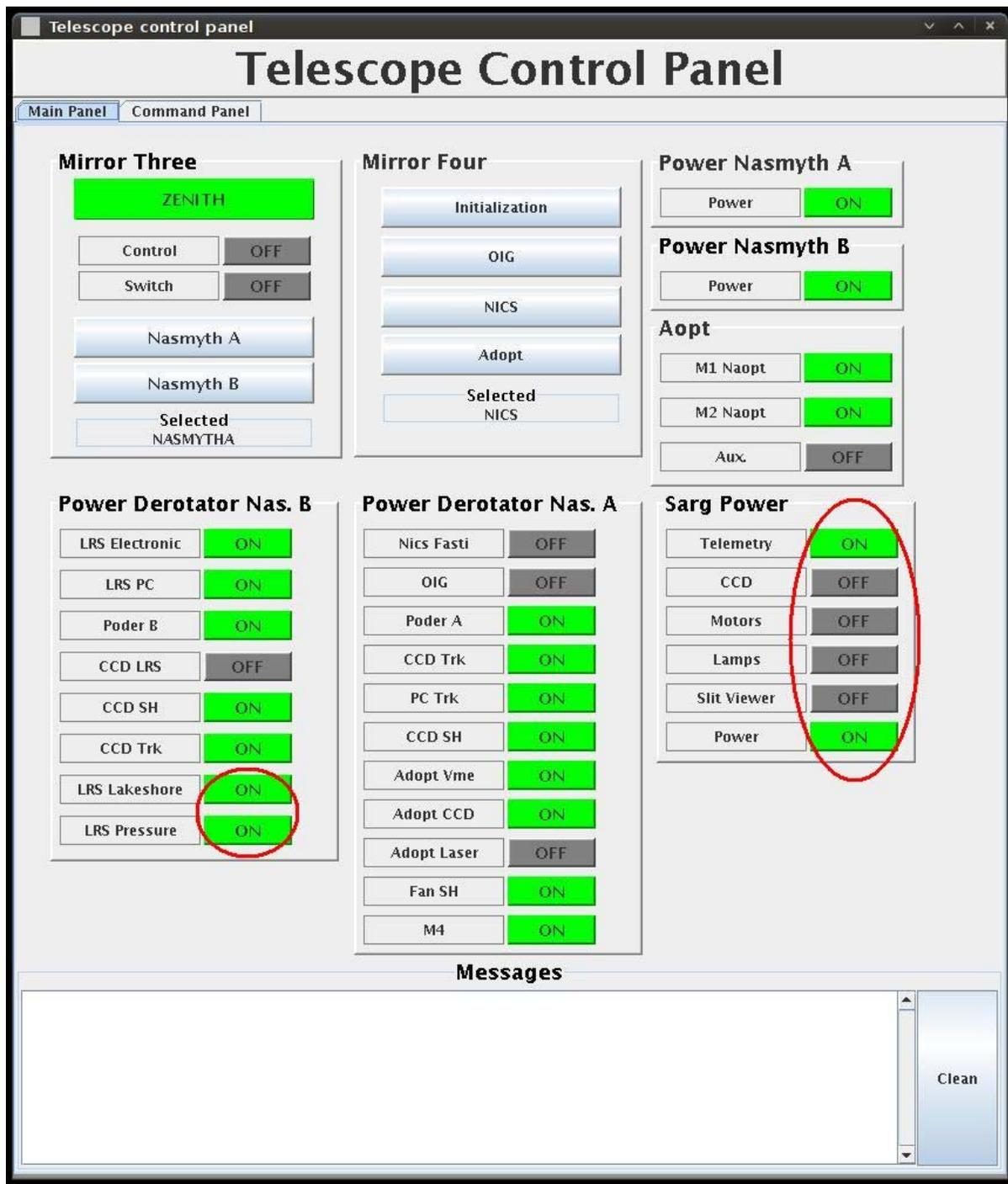
Figure 3 - Click on the red circled button to switch 'ON' all the sections of SARG. The Telescope Control Panel interface program runs on the WLBUILD computer.
