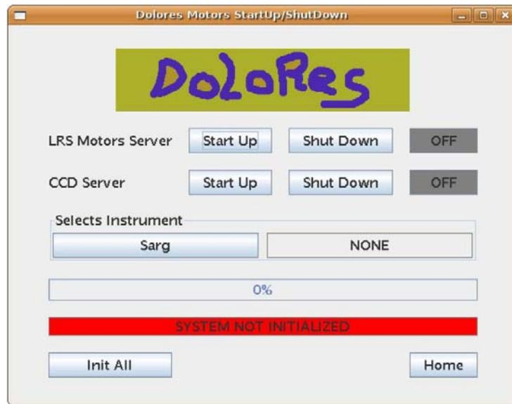
Figure 5 - A double click on the "Dolores Motors Start Up" icon on the LRS linux PC desktop will open this panel.
