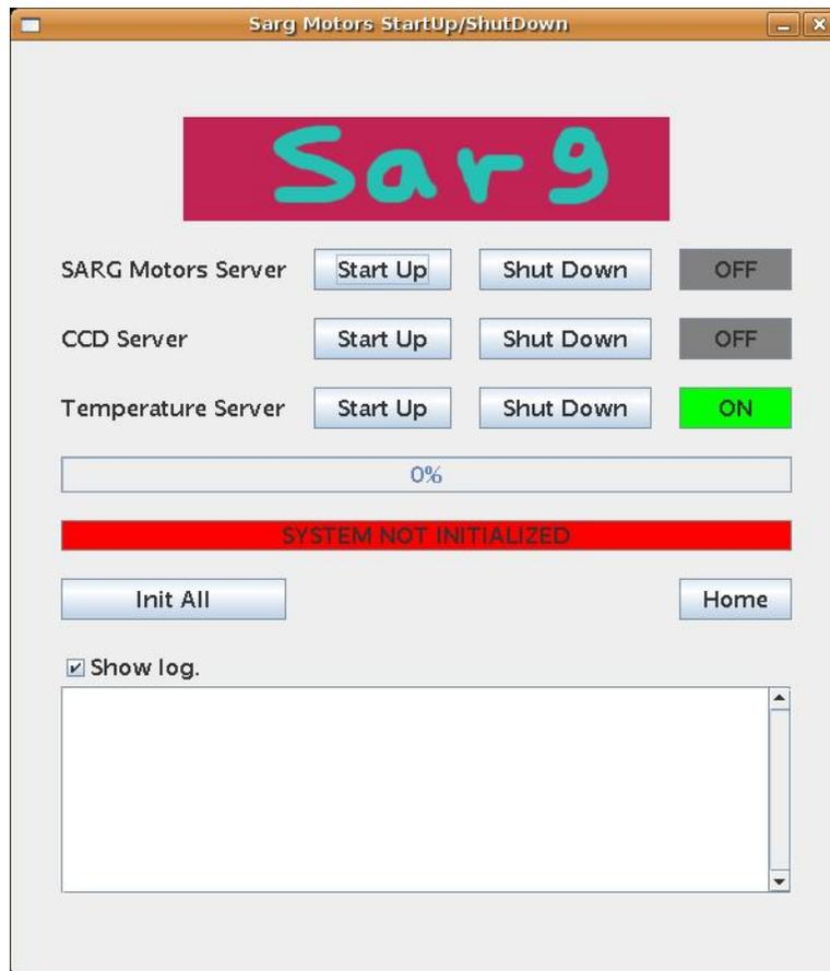
Figure 6 - A double click on the "Sarg Motors Start Up" icon on the LRS linux PC desktop will open this panel. Actions to be done here are described in the text.
