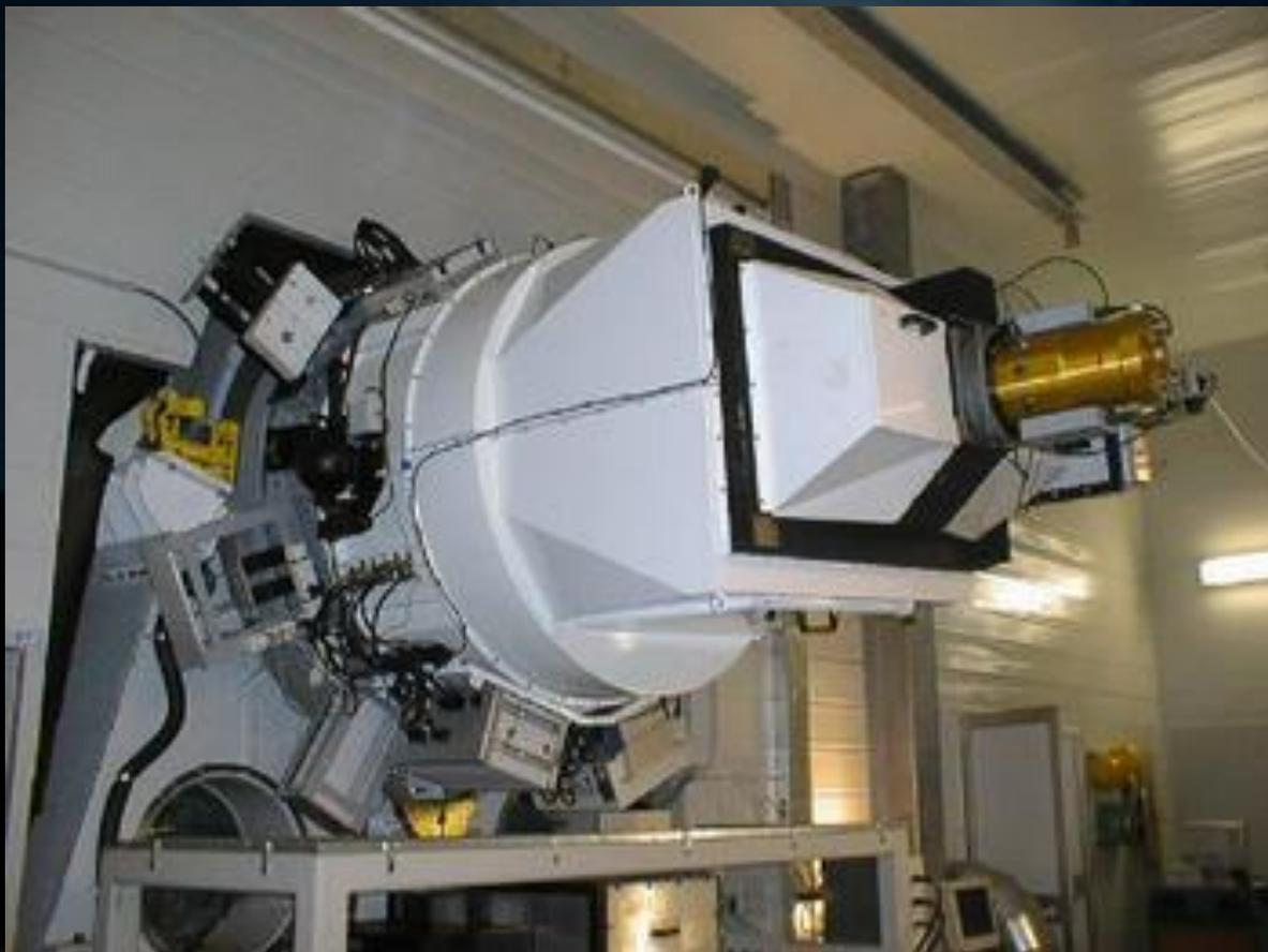
Low resolution spectrograph and camera installed at the Nasmyth B focus of the TNG
