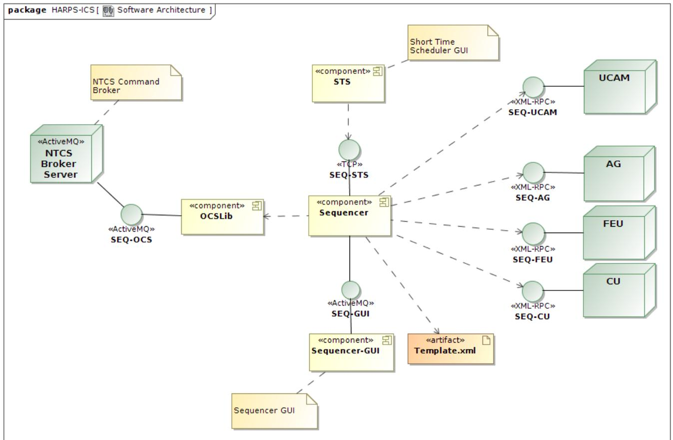
Figure 10 - The HARPS-N software architecture (not upgraded)
