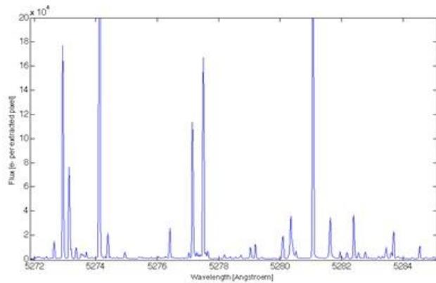
Figure 17 - Portion of the extracted ThAr spectrum order
