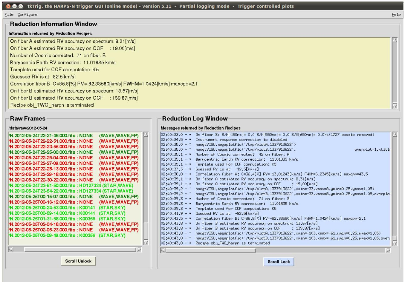
Figure 16 – Screenshot of the data-reduction trigger
