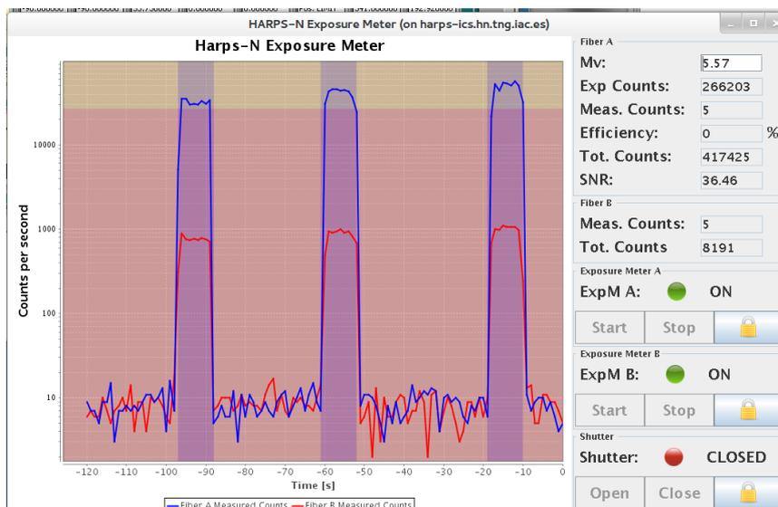
Figure 9 - Exposure meter GUI
