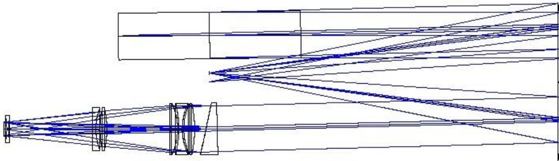
Figure 2 - Optical layout of the spectrograph
