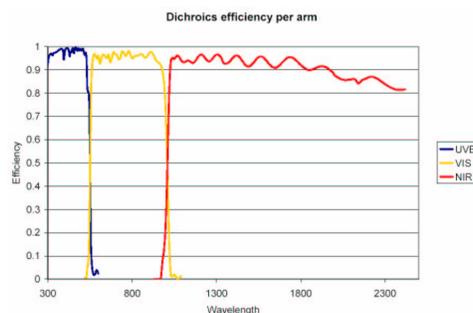
**Fig. 4.** Efficiency of the X-shooter dichroics
