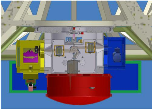
**Fig. 2.** X-shooter general layout. The backbone, shown attached to the Cassegrain focus of the VLT, contains the pre-slit optics pre-processing and despatching the light into the UV (left), the VIS (right) and the IR (bottom) arms.
