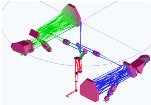
**Fig. 3.** X-shooter 4C Optical design (NIR arm not shown).
