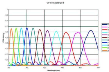
**Fig. 5.** Computed efficiency of the UV arm Echelle.
