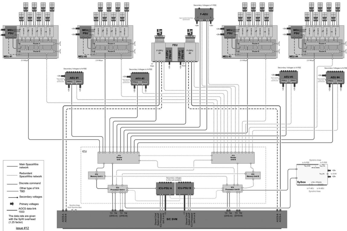
Figure 2. PLATO Data Processing System (DPS) overview.
