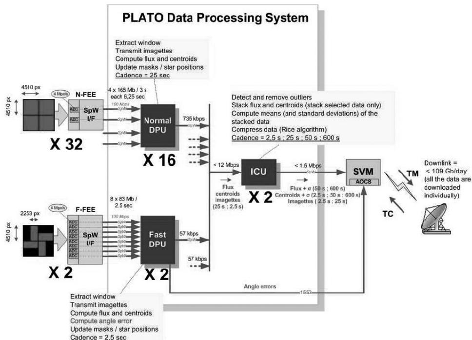
Figure 1. Overview of the PLATO data processing system architecture and of the data flow rates.
