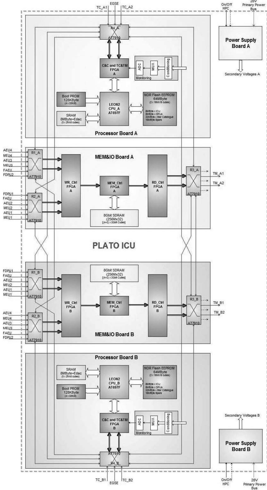
Figure 3. PLATO ICU overall HW architecture.
