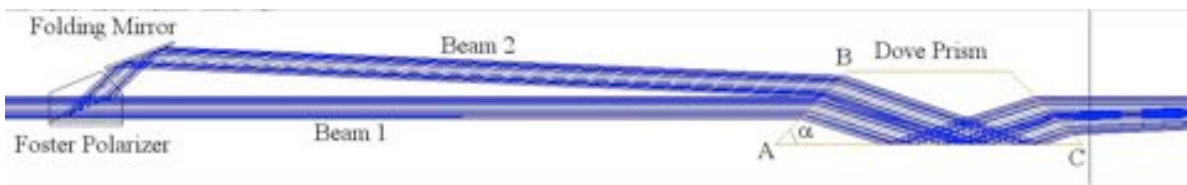
Figure 3. To match the very separated (16 mm) HARPS-North fibers on the focal plane, a Foster prism combined with a Dove prism have been selected. The fine M5 tip-tilt mirror integrated in the HARPS-North Front End Unit (FEU) will fix the two spots on them. A \lambda/2 retarder (top-right) has been glued on the 45° exit face of the Foster prism to maximize the reflection onto the mirror. To fix the polarimeter optical axis on the sky reference system despite the Alt-Azimuth mount, the Foster prism rotates as the parallactic angle. The emerging ordinary and extraordinary beams go through a Dove prism that properly anticounter-rotates to feed HARPS-North fibers.
