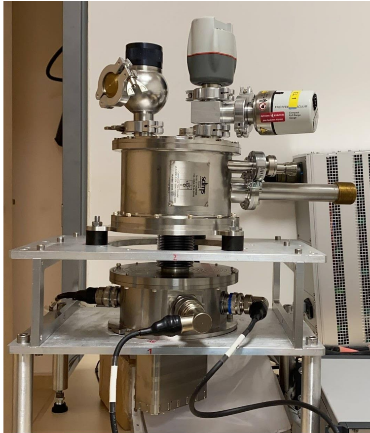
Figure 4 - Camera housing and CFC mounted in the test bench
